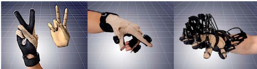
Abbildung 2.6: v.l.n.r. CyberGlove II, CyberTouch, CyberGrasp [Cyb14]
